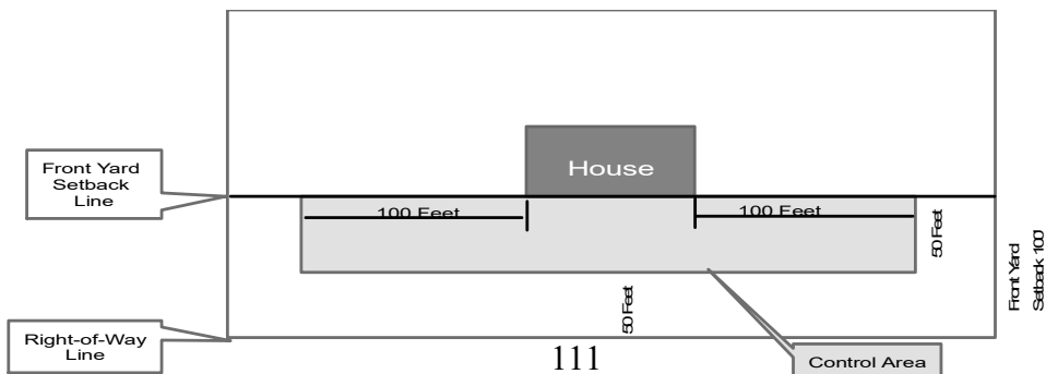
Figure 1608.3 Controlled Area Illustration
